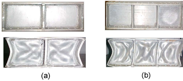
Fig. 7 State of test specimens before and after the testing: (a) two paneled specimen and (b) three-paneled specimen
