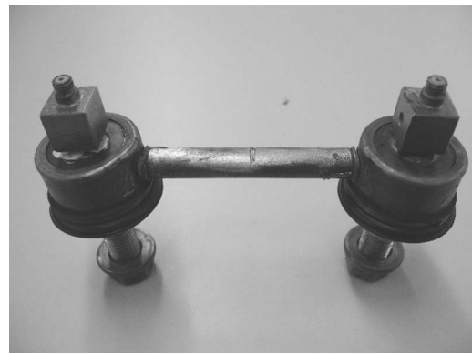
Fig. 6 Accelerometers attached to the ends of sway bar link
