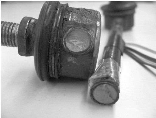
Fig. 12 Fatigue failure of sway bar link under constant amplitude cyclic loading
