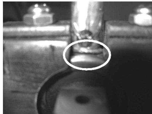
Fig. 8 Initial circumferential crack in sway bar link under cyclic loading
